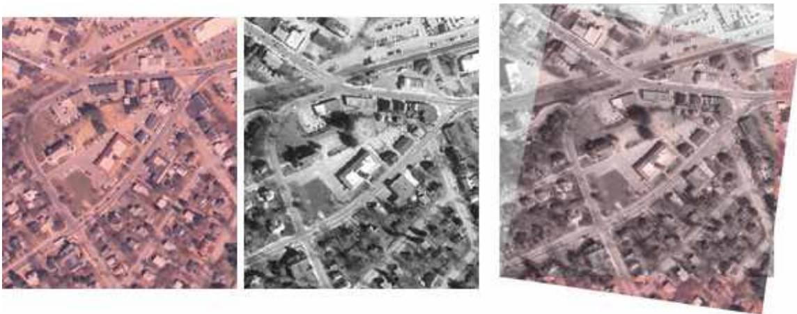
Figure 3.12: Image registration assuming an infinite amount of space [30]
